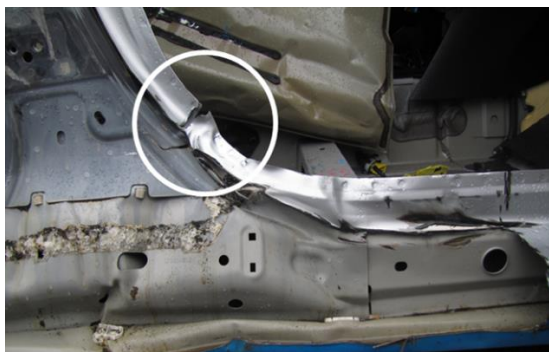
Rupture of a B-Pillar.
