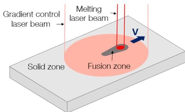
*Control of thermal gradient during fabrication*
