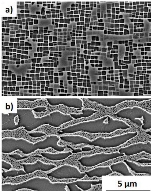
Microstructure of CMSX-4SLS (1 at. % of Re)
