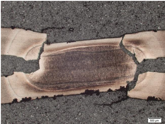
Optical Microscope cross sectional view of a fractured Resistance Spot Weld
